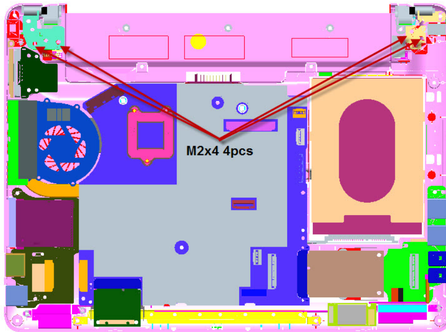
Figure 4-8-8 Remove the hinge screws
